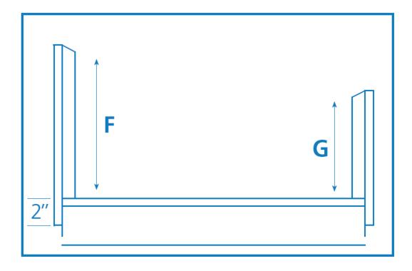
Notice the angle made by the 2" x 4" vertical bracing and the 2" overlap on the base.
