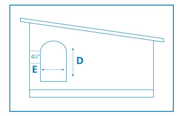
The roof is made from 3/4" plywood and has a 3" overhang on the high side and the low side. It has a 6" overhang on the door side and a 3" overhang on the back.
